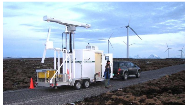
Figure 6. Merlin radar system for investigating bird flight in the wind power plant. Photo: K. Bevanger
