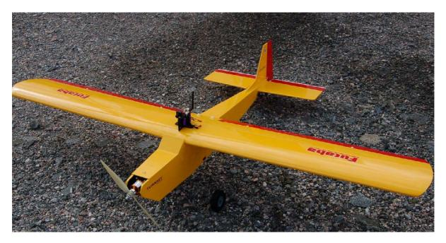
Figure 36. Model aircraft with video camera and transmitter. Photo: Pål Kvaløy.
