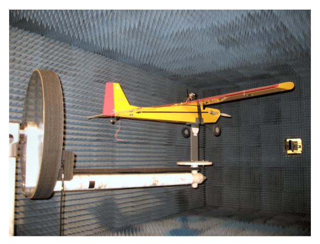
**Figure 38.** Model aircraft used as test target mounted on the swivelling table on the measurement tower in the anechoic chamber. The radar antennas are in the window to the right in the picture. Photo: Yngve Steinheim.
