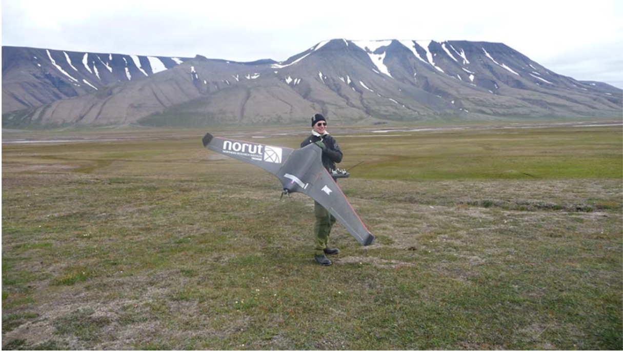
Figure 2. Field campaign using the Crywing micro UAS in surveying of the vegetation in the Adventdalen on Svalbard.
