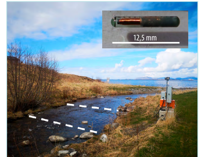
The PIT antenna at the Hegg River entrance which continuously monitors the out- and return-migration of sea trout. (Inset - a 12.5 mm PIT tag)
