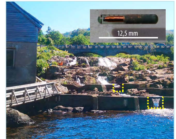
The PIT antenna at the Oselva river mouth which continuously monitors the out- and return-migration of sea trout. (Inset - a 12.5 mm PIT tag)
