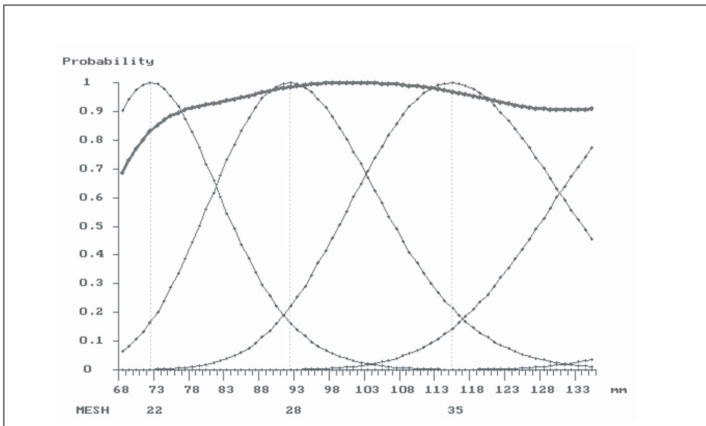
**Figure 5.11** Gill net selectivity for *Pharyngochromis acuticeps* for different mesh sizes from 22 mm to 45 mm (thin lines) and combined estimated selectivity curve for all mesh sizes (thicker line).
