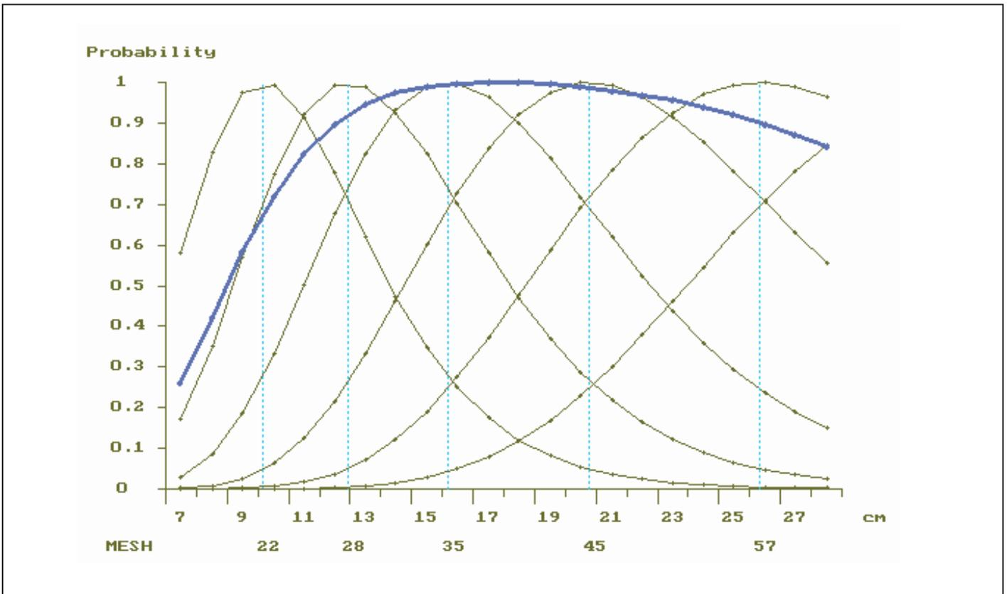
**Figure 5.9** Gill net selectivity for *Schilbe intermedius* for different mesh sizes from 22 mm to 57 mm (thin lines) and combined estimated selectivity curve for all mesh sizes (thicker line).
